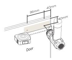
Place masking tape on both sides of the door where holes will be drilled to avoid chipping. Pre-drill using 4.5mm drill bit
