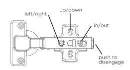
Clip the door onto the hinge plates.
