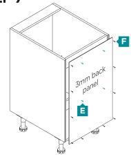
**note:** The white side of the back panel should face inside the cabinet.
