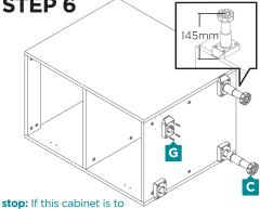
be installed at the end of the run refer to the kickboard instructions now on the correct placement of the feet.
