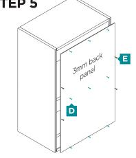
**note:** The white side of the back panel should face inside the cabinet.
