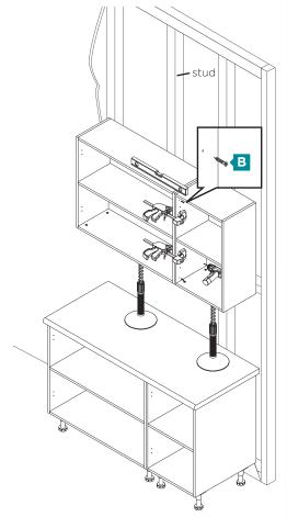
Check cabinets are level then clamp together. Pre-drill using 2mm drill bit and attach cabinets together. **STEP 12**
