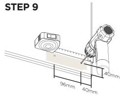
Place masking tape on both sides of the door where holes will be drilled to avoid chipping. Pre-drill using 4.5mm drill bit
