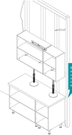
Caution: Please ensure all cabinets are screwed into your timber stud wall using a minimum of 65mm timber screws. If attaching to concrete, brick, steel or any other substrates seek advice from your hardware specialist.
