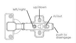
To align doors adjust marked screws.
