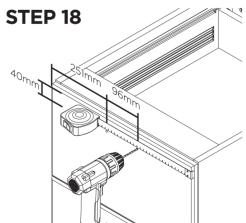
Place masking tape on both sides of the door where holes will be drilled to avoid chipping. Pre-drill using 4.5mm drill bit.
