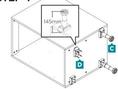
stop: If this cabinet is to be installed at the end of the run refer to the kickboard instructions now on the correct placement of the feet.
