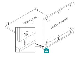
note: Make sure the pre-drilled holes for the adjustable feet are facing outwards.
