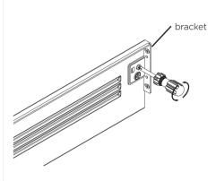
Remove bracket from metal sided drawer by releasing screw.
