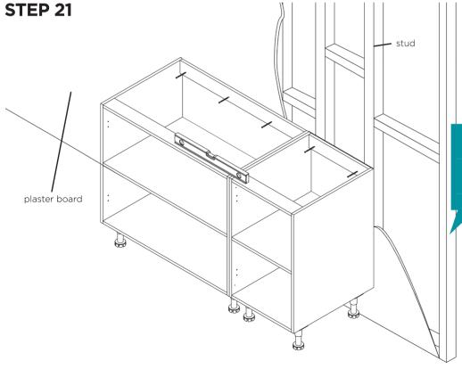
Caution: Please ensure all cabinets are screwed into your timber stud wall using a minimum of 65mm timber screws. If attaching to concrete, brick, steel or any other substrates seek advice from your hardware specialist.
