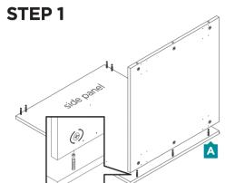
**note:** Make sure the pre-drilled holes for the adjustable feet are facing outwards.
