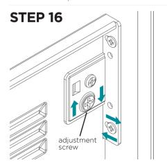
Drawer fronts can be adjusted up and down via the adjustment screw, and left and right via the elongated holes in the bracket.
