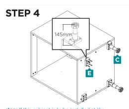
**stop:** If this cabinet is to be installed at the end of the run refer to the kickboard instructions now on the correct placement of the feet. Set the height of the adjustable feet to 145mm to suit the kickboard.
