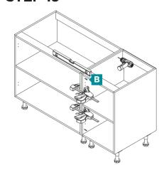
Check cabinets are level then clamp together. Pre-drill using 2mm drill bit and attach cabinets together.
