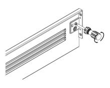
Remove bracket from metal sided drawer by releasing the screw.
