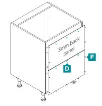
note: The white side of the back panel should face inside the cabinet.
