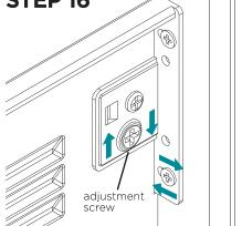
Drawer fronts can be adjusted up and down via the adjustment screw, and left and right via the elongated holes in the bracket.
