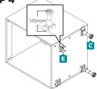
stop: If this cabinet is to be installed at the end of the run refer to the kickboard instructions now on the correct placement of the feet. Set the height of the adjustable feet to 145mm to suit the kickboard.
