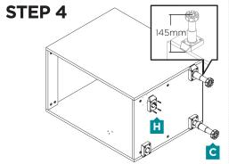
**stop:** If this cabinet is to be installed at the end of the run refer to the kickboard instructions now on the correct placement of the feet.
