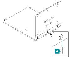
**note:** Make sure the pre-drilled holes for the adjustable feet are facing outwards.
