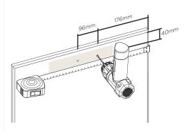
Place masking tape on both sides of the door where holes will be drilled to avoid chipping. Pre-drill using 4.5mm drill bit
