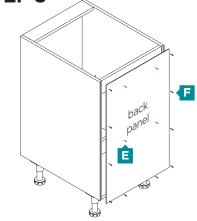
**note:** The white side of the back panel should face inside the cabinet.
