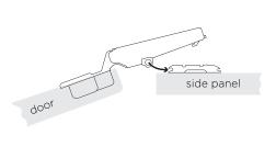
Clip the door onto the hinge plates.
