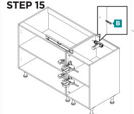
Check cabinets are level then clamp together. Pre-drill using 2mm drill bit and attach cabinets together.
