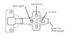
To align doors adjust marked screws.
