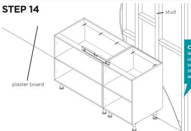
Caution: Please ensure all cabinets are screwed into your timber stud wall using a minimum of 65mm timber screws. If attaching to concrete, brick, steel or any other substrates seek advice from your hardware specialist.
