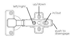
Clip the door onto the hinge plates.
