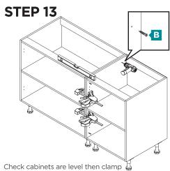
together. Pre-drill using 2mm drill bit and attach cabinets together.
