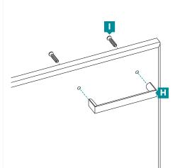
To align doors adjust marked screws.
