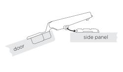
Clip the door onto the hinge plates.
