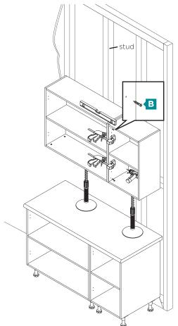
Check cabinets are level then clamp together. Pre-drill using 2mm drill bit and attach cabinets together.
